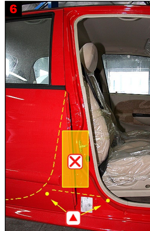
6 B-pillar: Treat via 2 drilled holes. No treatment upwards because of safety belt
