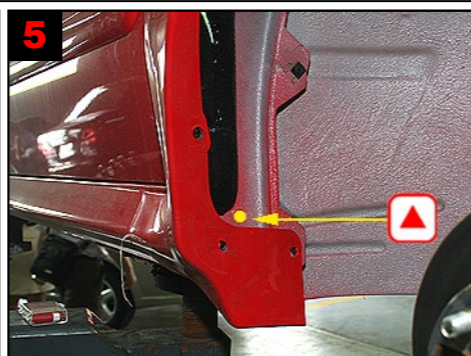
5 Wheel arch front/panel: Treat via 1 drilled hole.
