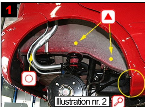
1 Wheel arch rear/ longitudinal member: Treat via 2 drilled holes as well as via existing hole. Panel: See fig 2.
